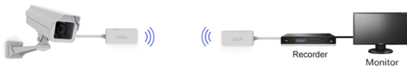
Solution Two Camera 1,2,3---Bridge Bridge---Recorder---Monitor
