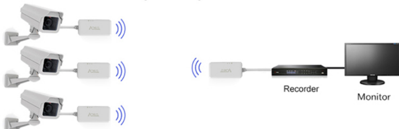
Solution Three Camera 1,2,3---Switch-Bridge Bridge---Recorder---Monitor
